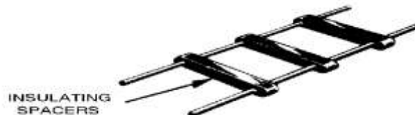
Figure 2. - Parallel two-wire line
